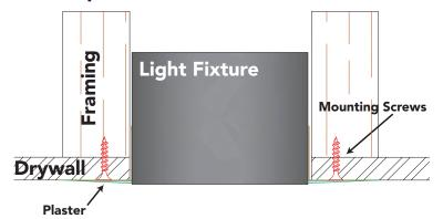
**Framing Required!** Build framing on either side of light fixture.
