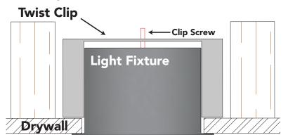
Twist Clip Mounting: Specialized clip secures light fixture to drywall.
