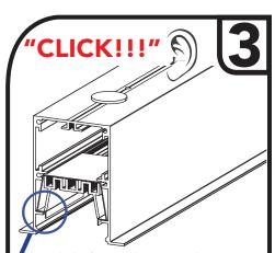
Drop light fixture down into the opening that was created when ceiling structure was built. Make sure light fixture sits flat, and grid brackets go over grid structu
