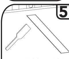
Use compound knife for a smooth finish. Sand, paint, and finish all drywall work before removing contractor's tape.
