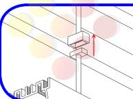
Before inserting inner-channel be sure to make electrical connections using the provided connectors. Connection should be secure.
