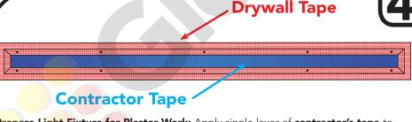
Prepare Light Fixture for Plaster Work: Apply single layer of contractor's tape to channel opening (if lens removed), or lens. Do not use multiple layers of tape. If covering channel opening, make sure to cover area where lens snaps into place.
